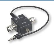
The low current adapter is used to calibrate shunts at currents levels of 2 A or less. It connects together the current source and two shunts for calibration measurements. This adapter mates with N-type connectors to the shunts and a dual banana connection to the source. In this configuration, a certified or reference shunt is connected in series with a shunt that is being calibrated, which in turn are in series with a current source.
